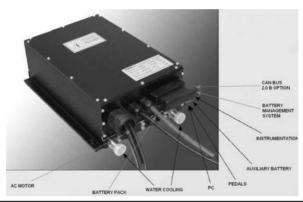
FIGURE 9-33 MES-DEA TIM Series TIM 300 (30 kW), TIM 400 (50 kW), TIM 600 (100 kW), and TIM 900 (200 kW) view and connection description. (www.metricmind.com.)
