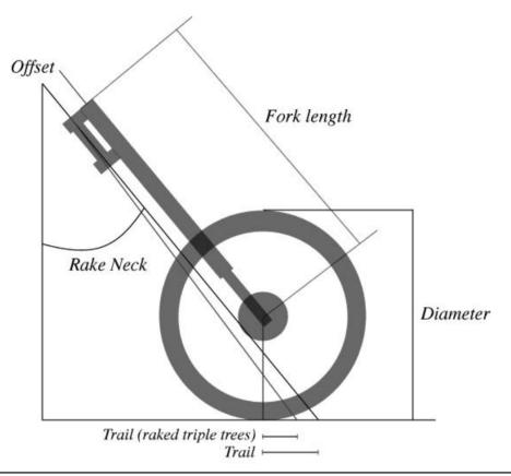
FIGURE 5-6 Example of the effect of a change in rake angle on trail. (www.carbibles.com/suspension\_bible\_bikes.html.)
