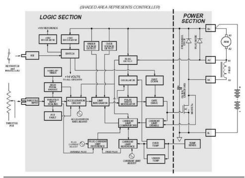
FIGURE 9-4 Controller logic. (Courtesy of Curtis Instruments, www.curtisinst.com.)
