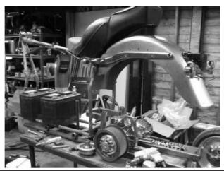
FIGURE 13-7 Fitting the transmission to the swingarm.
