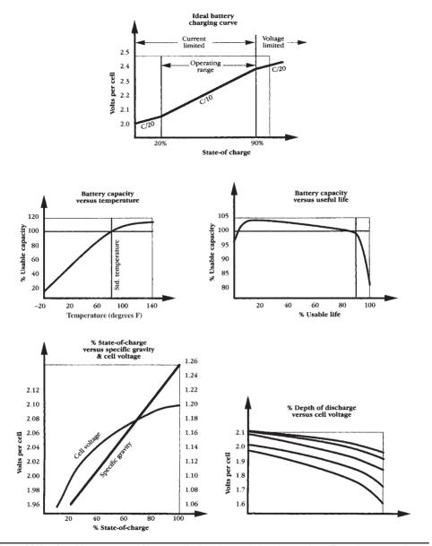
FIGURE 10-1 Graphic summary of battery discharging and charging cycles. (From *Build Your Own Electric Vehicle*, Table 9-1, p. 216.)
