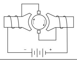
FIGURE 8-11 Drawing of a field coil.
