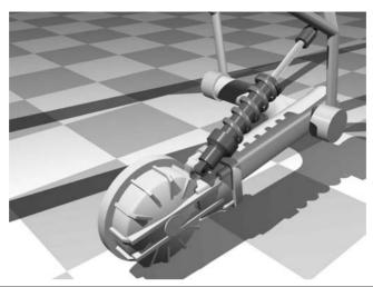
Figure 5-19 Monolever rear suspension system. (www.carbibles.com/suspension\_bible\_bikes. html.)
