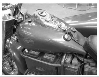
FIGURE 11-12 Electra Cruiser prototype 2 tank and gauges.
