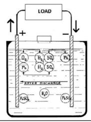
Figure 7-19 Discharging reaction. (www.powerstream.com/1922/battery\_1922\_WITTE/batteryfiles/chapter11.htm.)
