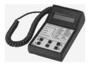
Figure 9-19 ZAPI digital programming console. (www.zapi.co.za/zapi/images/programmingconsole.jpg.)
