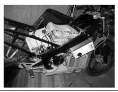
FIGURE 4-2 Electrocat batteries and electric motor. (evahakansson.se.)
