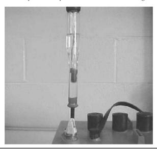
FIGURE 7-21 Glass tube hydrometer measuring specific gravity in a battery cell. (www2.tech. purdue.edu/at/courses/aeml/airframeimages/hydrometerinbatt.jpg.)
