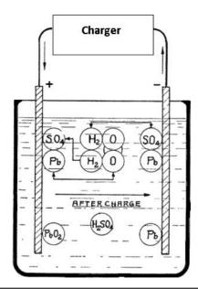
Figure 7-20 Charging reaction. (www.powerstream.com/1922/battery\_1922\_WITTE/batteryfiles/chapter11.htm.)
