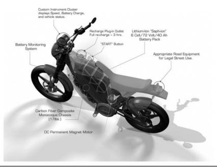
FIGURE 4-7 Specifications of the Enertia bike. (enertiabike.com.)
