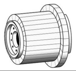
Figure 8-8 CAD drawing of a simple commutator.
