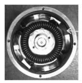
Figure 8-10 Field pole in the housing of a series motor.
