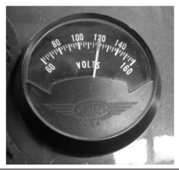
FIGURE 11-8 Voltmeter used on the Electra Cruiser. (www.westach.com/gauge\_images/2C6-30.gif.)
