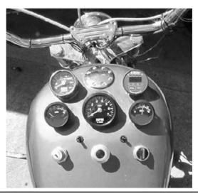
FIGURE 11-1 Electra Cruiser prototype 1 tank gauge layout.
