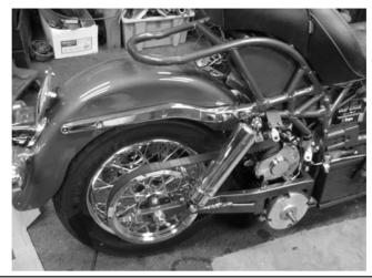
FIGURE 13-15 Cruiser swingarm and drive belt.
