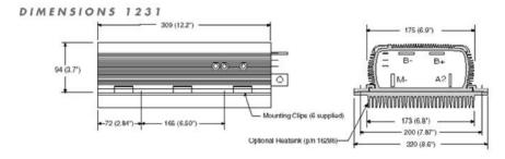
**Figure 9-8** Dimensions for Models 1221 and 1231. (www.curtisinst.com/index.cfm?fuseaction=cProducts.DownloadPDF&file=50003%5F1221C%2D1231C%5FRevD%2Epdf.)
