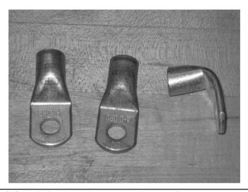
FIGURE 12-10 2/0 terminal ends used to connect to the controller or motor.
