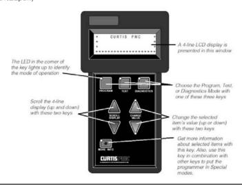
**FIGURE 9-17** Curtis programmer. (www.curtisinst.com/index.cfm?fuseaction=cProducts. dspProductCategory&catID=7.)
