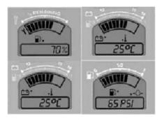
Figure 11-7 Curtis enGage II dual-function display examples. (www.curtisinst.com/index. cfm?fuseaction=cProducts.dsplnstrumentation.)
