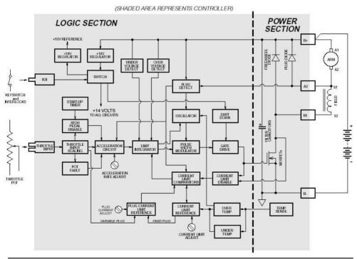
FIGURE 9-12 Typical block diagram for Curtis Model 1209B/1221B/1221C/1231C controllers. (www.curtisinst.com)
