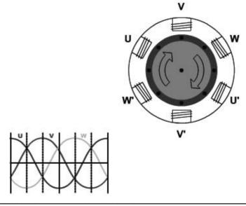
Figure 8-21 Ac induction motor rotating showing phases.
