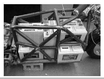
FIGURE 13-16 Fitting 10 Group 27 batteries in prototype 1.
