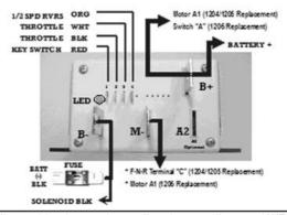
Figure 9-24 Typical Alltrax wiring layout. (www.alltraxinc.com/images/AXE-Wire-Diagram.gif.)
