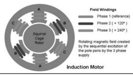
FIGURE 8-26 Three-phase ac motor.
