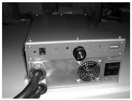
FIGURE 10-8 Manzanita Micro PFC-20, an extremely versatile battery charger. (From *Build Your Own Electric Vehicle*, Figure 9-4, p. 219.)
