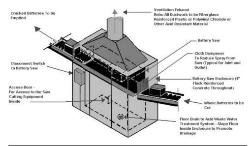
Figure 7-29 Battery saw used in recycling batteries. (www.osha.gov/SLTC/etools/leadsmelter/popups/batterysaw\_popup.html.)
