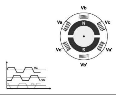
FIGURE 8-20 Ac induction motor with a permanent magnet armature showing phases.
