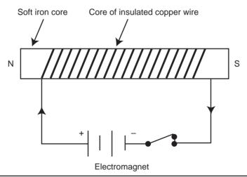
FIGURE 8-4 Simple electromagnet.
