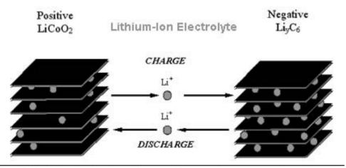
Figure 7-10 Lithium-ion electrolytes. (Courtesy of Electropaedia, www.mpoweruk.com/images/swingcell.gif.)
