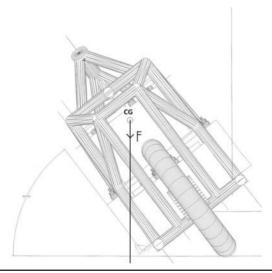
FIGURE 6-3 Bike center of gravity.
