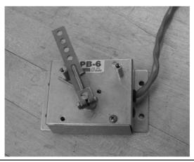
FIGURE 12-6 Curtis PB-6 5-k $\Omega$  potentiometer.
