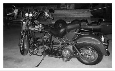
FIGURE 13-4 Prototype 2 Electra Cruiser ready for batteries.
