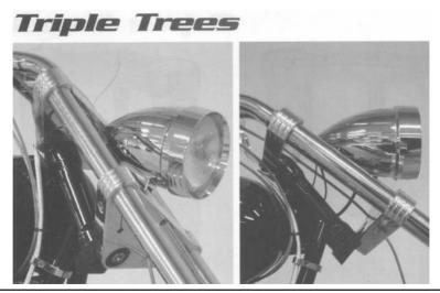
Figure 5-8 Raked triple-tree example. (Courtesy of Custom Chrome, www.customchrome.com.)
