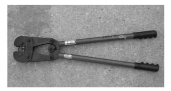
FIGURE 12-9 Heavy-duty crimping tool.
