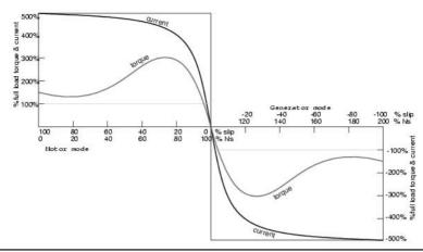
FIGURE 8-27 Basic ac induction motor and regenerative motor curve. (http://electojects.com/motors/tesla-induction-motors-4.htm.)
