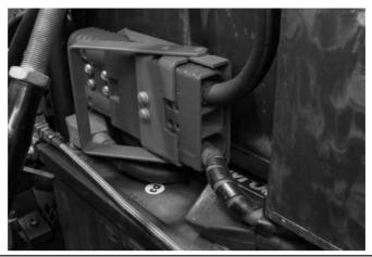
FIGURE 12-2 Quick disconnect on the Electra Cruiser.
