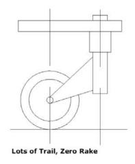
FIGURE 5-7 The castor on a shopping cart in relation to trail and rake.
