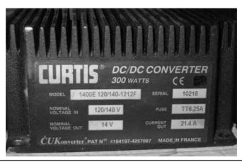
FIGURE 11-16 Curtis dc-to-dc converter back panel.
