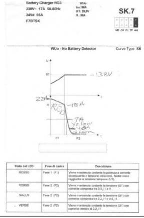
Figure 10-7 Charging profile for NG3 220-V ac/120 V dc unit.
