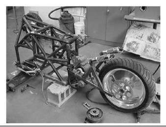
FIGURE 13-8 Transmission placed on prototype 1 swingarm.
