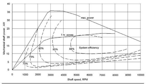
Figure 8-23 Combined efficiencies of the Simovert ac inverter at 130 V dc input. (Courtesy Metric Mind Engineering, www.metricmind.com.)
