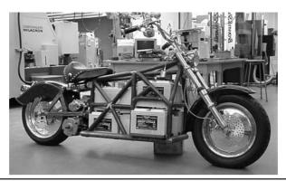
FIGURE 5-14 Prototype of Electra Cruiser loaded with 560 lb (254 kg) of batteries.
