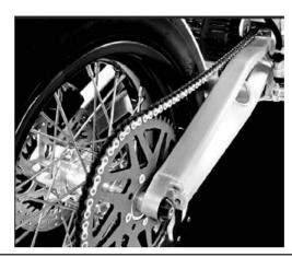
FIGURE 13-9 ZERO electric motorcycle chain drive. (www.zeromotorcycles.com/gallery.php.)
