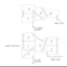
FIGURE 13-21 Battery wiring, top and bottom levels.
