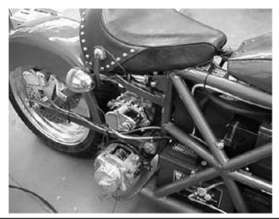
FIGURE 13-13 Rear mounting bracket for the dc motor.
