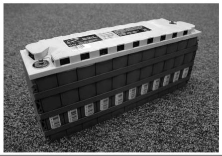
Figure 7.3 Ovonic EV1 battery in an S-10 pickup. (Courtesy of Mike Anzalone of Long Island Electric Auto Association [LIEAA].)
