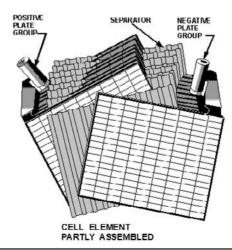
Figure 7-12 Illustration of battery plates with separators. (www.tpub.com/neets/book1/chapter2/2-10.gif.)
