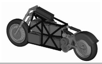
FIGURE 1-6 Three-dimensional (3D) drawing of the first prototype produced in AutoCAD.
