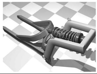
FIGURE 5-16 Monoshock H-style swingarm rear suspension. (www.carbibles.com/suspension\_bible\_bikes.html.)
