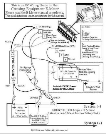
FIGURE 11-3 Link 10 wiring. (www.xantrex.com.)
