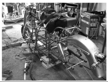
FIGURE 13-6 Prepping the Cruiser frame for cleaning and more welding.
