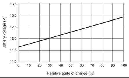
Figure 7-23 Graph of voltage versus capacity.
