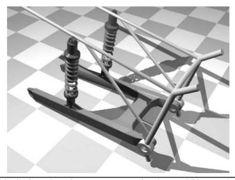
Figure 5-15 Twin-shock regular swingarm rear suspension. (www.carbibles.com/suspension\_bible\_bikes.html.)
