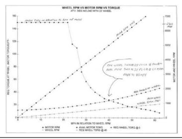
**FIGURE 6-10** Wheel rpm versus motor rpm versus torque on a 0-degree incline.
