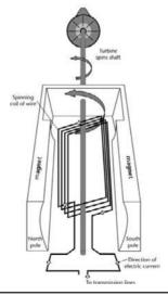
FIGURE 2-3 Turbine generator. (www.eia.doe.gov/kids/energyfacts/sources/electricity.html.)
