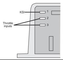
FIGURE 9-14 Curtis Model 1221/1231 series potbox connections. (www.curtisinst.com/index. cfm?fuseaction=cProducts.DownloadPDF&file=50003%5F1221C%2D1231C% 5FRevD%2Epdf.)
