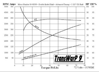
FIGURE 8-15 Nine-inch motor curves. (Courtesy of NetGain Motors, Inc.)
