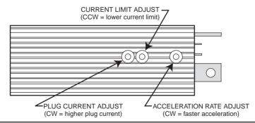
Figure 9-9 Basic adjustment location. (www.curtisinst.com/index.cfm?fuseaction=cProducts. DownloadPDF&file=50003%5F1221C%2D1231C%5FRevD%2Epdf.)
