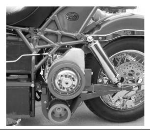
FIGURE 13-14 Clutch basket and belt configuration.
