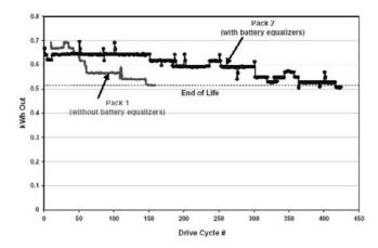
Figure 10-14 PowerCheq cycle life with balancing module. (Courtesy of Power Designers USA, http://powerdesignersusa.com/powercheq\_faq.htm.)
