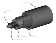
FIGURE 8-6 Three-dimensional (3D) representation of basic motor components.
