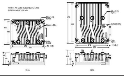
FIGURE 9-28 Curtis Model 1236/38AC controller dimensions. (www.curtisinst.com/index.cfm? fuseaction=cProducts.DownloadPDF&file=50095%5F1236%2D1238%5FRevG1%2E pdf.)
