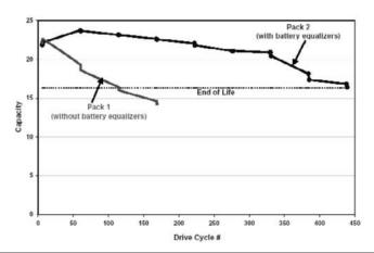
Figure 10-15 PowerCheq capacity life with balancing module. (Courtesy of Power Designers USA, http://powerdesignersusa.com/powercheq\_faq.htm.)
