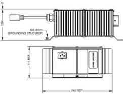
FIGURE 10-10 Curtis Model 1621 battery charger dimensions. (www.curtisinst.com/index. cfm?fuseaction=cProducts.BatteryChargers.)
