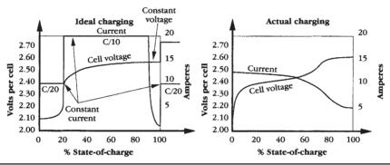
FIGURE 10-2 Graphic summary of battery discharging and charging cycles. (From *Build Your Own Electric Vehicle*, Figure 9-3, p. 211.)
