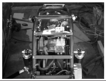
FIGURE 13-18 Controller and components packed tightly in the underseat area.
