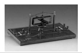
Figure 8-2 Example of an early dc motor. (http://upload.wikimedia.org/wikipedia/en/3/34/World's\_first\_electric\_motor\_Jedlik's\_motor\_(1828).jpg.)
