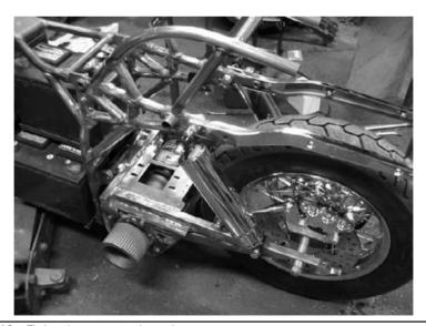
FIGURE 13-12 Fitting the motor to the swingarm.
